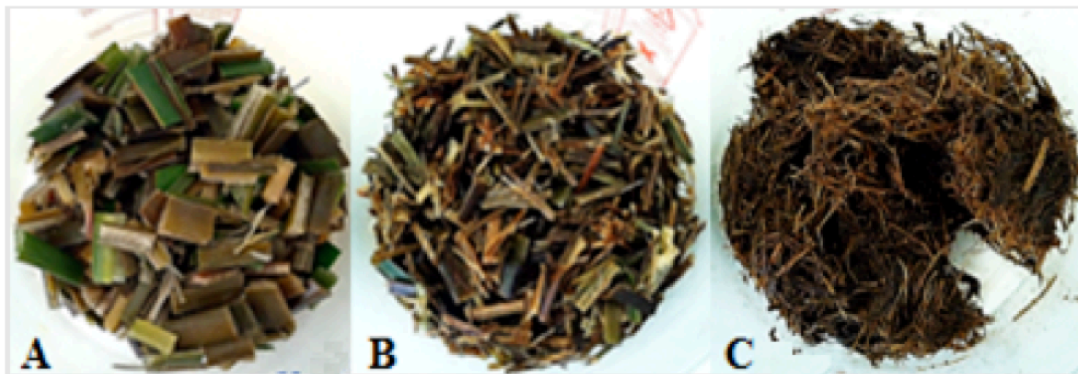
Figure 1. Solid phase of narrow-leaved cattail after pretreatment conditions at 140 °C – 5 min (A), 170 °C – 5 min (B) and 210 °C – 5 min (C).
