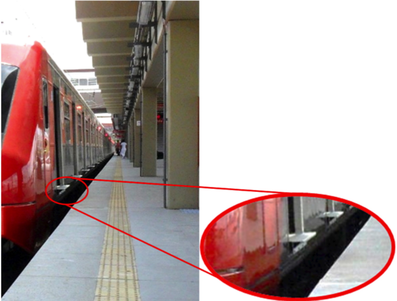
Figure 1 Device to reduce the space between the subway car and the platform
